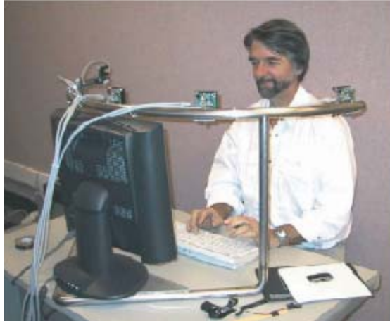
Figure 2.7: HP's Coliseum project tries to keep a large enough sensor array to capture several users and having a small display, sacrificing the sight line between the users. (image courtesy of [27]).
