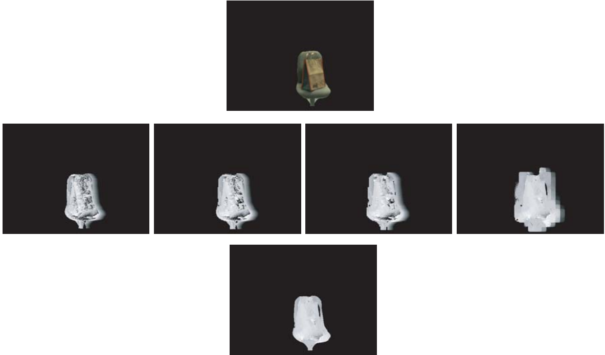
Figure 3.7: In the top row we can see the segmented object. In the middle row we can see from left to right the disparity-map with 0,1,2 and 4 mipmap levels. The bottom image represents the disparity-map with 4 mipmap levels cut out by the segmentation mask.
