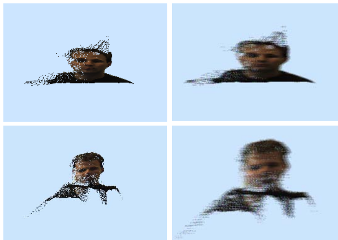
Figure 4.12: Rendering results with GL_POINTS of size 1.0. On the left side we can see the view of the virtual camera in the middle. On the right side the inter-zigged image for the auto-stereoscopic display. On top we look directly into our stereo camera pair and have the virtual cameras in the same spot. On the bottom we look directly into the display and the virtual cameras are aligned in a manner that a sight line to the conversational partner is built up.
