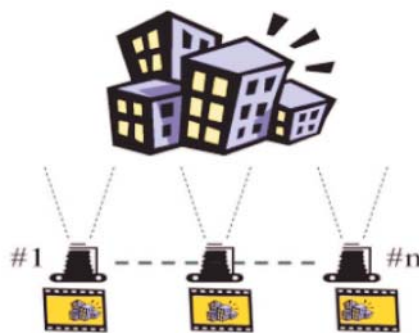
Figure 2.9: We need 9 different views from cameras that are aligned on one horizontal line to create our 3D image. (image courtesy of [24]).
