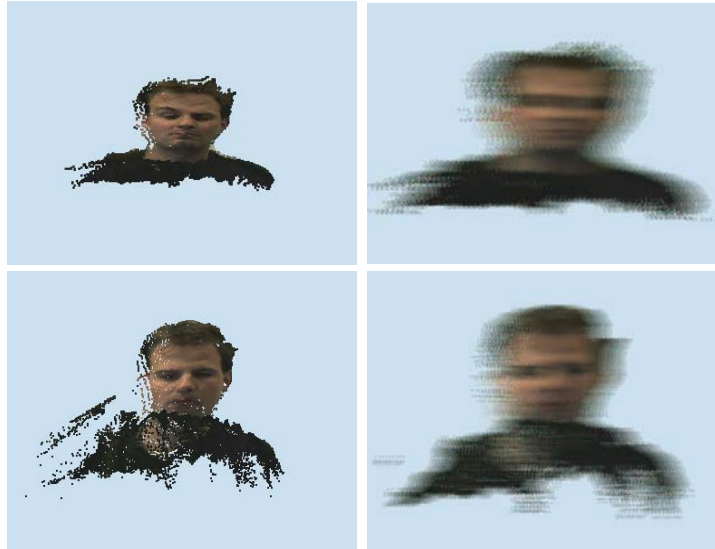
Figure 4.14: Rendering results with GL_POINTS of size 1.5. On the left side we can see the view of the virtual camera in the middle. On the right side the inter-zigged image for the auto-stereoscopic display. On top we look directly into our stereo camera pair and have the virtual cameras in the same spot. On the bottom we look directly into the display and the virtual cameras are aligned in a manner that a sight line to the conversational partner is built up.
